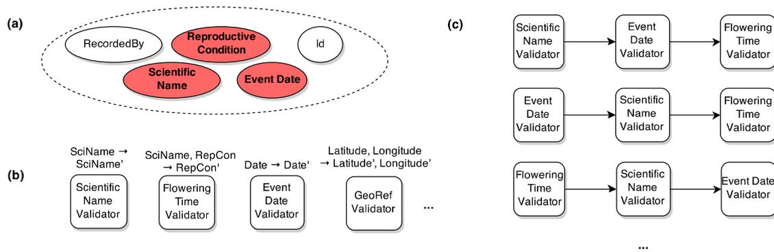
**Figure 4.** Example showing how the design engine works: (a) an input data schema and a set of data fields (highlighted) that need to be curated, (b) an actor library, and (c) some of the candidate workflows generated by the design engine.
